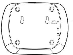
WiFi Reset switch: press and hold down for 10S then release, the blue WiFi indicator will go off and go on again, WiFi setting will be factory reset.
